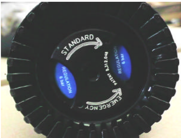
Regulated to 6 bar standard pressure (Midmatic and Midforce)
